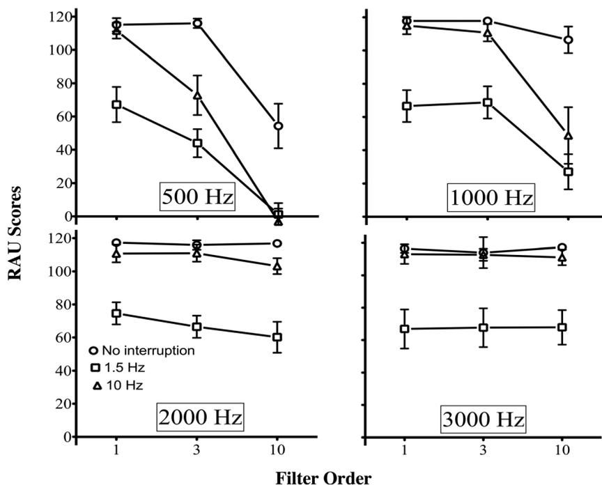
Fig. 1. The mean RAU scores shown as a function of the filter order. The panels show the results for different cut-off frequencies, and within each panel, the results are shown separately for different interruption conditions. The error bars denote the standard deviations.
